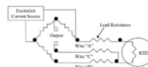
Gambar 4. 2 Rangkaian RTD PT100 (Suprianto, 2015)
