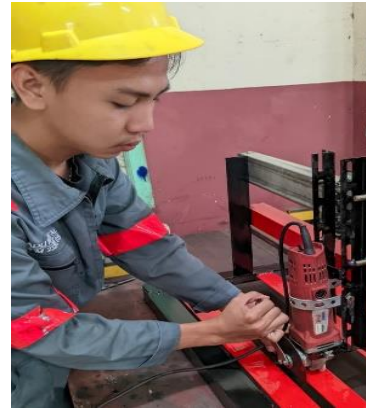
Gambar .3 Pengencangan mur mata gerinda (Ineer outer)
